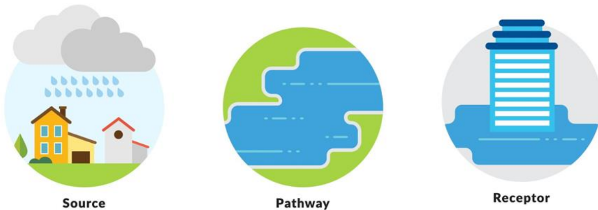
Figure 3-2 Source - pathway - receptor model
